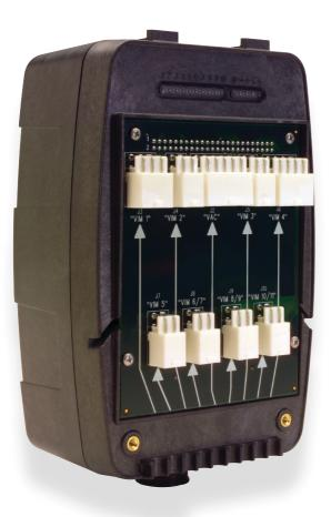
To create housings for asset tracking devices, a US-based manufacturer had long used fire-retardant PC with copper/ nickel metallization for EMI shielding. The OEM requirements were typical for this sort of device
