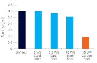
LNP FARADEX compounds' low volumetric loading of conductive filler results in near isotropic shrinkage properties very similar to the base thermoplastic the compounds are based on.
