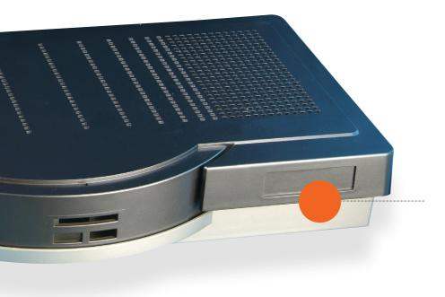
Designing this electronic housing to be made from LNP FARADEX NS0031 compound allowed the OEM to address their EMC requirements while eliminating a costly, time consuming and environmentally unfriendly multistep metallization coating process.
